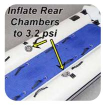
When transom is installed and all screws tightened, inflate the rear chambers.
