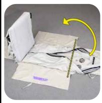
Lift open the last fold. Make a crease behind the valves and fold the bow onto the center of the bag.
