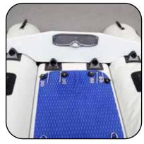
Start with floor grommets. Adjust transom board to align the holes.
