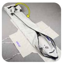
Fold the boat from the back (stern) towards the valves in the front (bow). Make a crease in the fabric about 3-feet from the end between the transom mounting grommets and the rod holders. Make the first fold on the crease.
