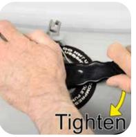
Press on center of valve tool with free hand to keep from breaking the teeth off the tool.
