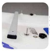
Fold the D-rings closest to the front of the boat outward. Place a washer over a bolt and run bolt up through D-ring.
