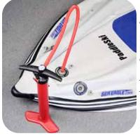
With valve stem in the up position, insert adapter, push down firmly and twist clockwise.
