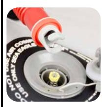
The pump hose has a **Recessed Valve Adapter** at one end. When ready to inflate the boat, push adapter firmly into valve and twist clockwise to lock
