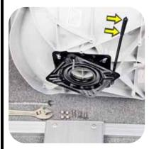
Turn seat on its side. Pull handle outward to unlock swivel and turn base so holes in the plates are offset as shown in the photo. Insert one screw in a slotted hole in the swivel.
