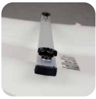
Place yoke bar over screws, secure with washer and knob.
