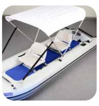
Attach the rear clips to the small D-rings behind transom. Attach front straps behind the yoke bar. Adjust and tighten straps by sliding the buckles.
