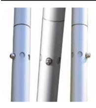
The additional holes in the shaft are for "feathering" the blades. Blades can be offset 45° from each other. This makes paddling into a stiff breeze easier as the blade that is not in the water will be able to slice through the wind with little resistance.
