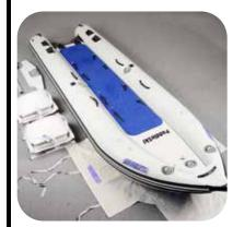
Remove transom, seats, yoke bar, rod holders, and canopy. Rod holder bases remain in place.
